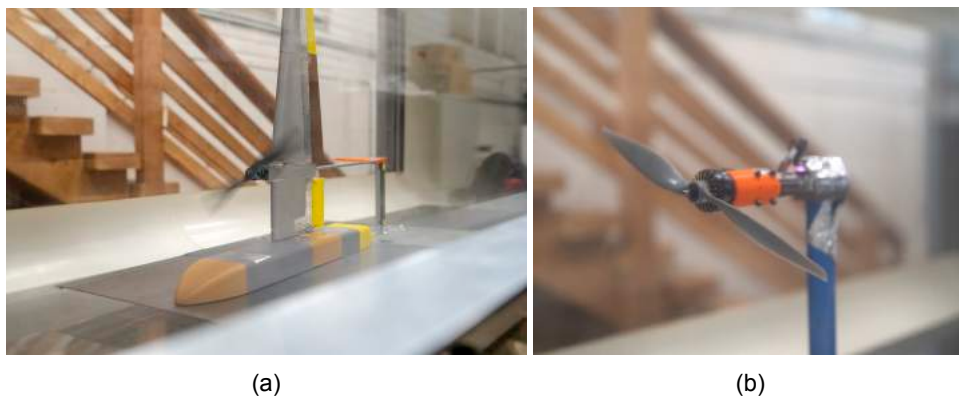
Figure 44: (a) Airframe half-body mounted vertically in wind tunnel and (b) motor-propeller propulsion test apparatus
