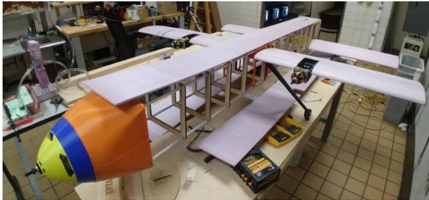
Figure 30: Aerodynamic Prototype Mid-Manufacturing
