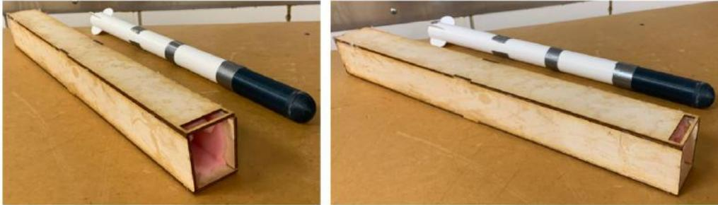
Figure 50: Sensor and Container Before and After Drop Test
