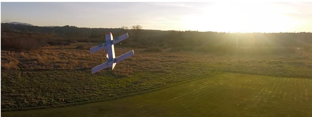
Figure 51: Aerodynamic Prototype in Sideslip Condition
