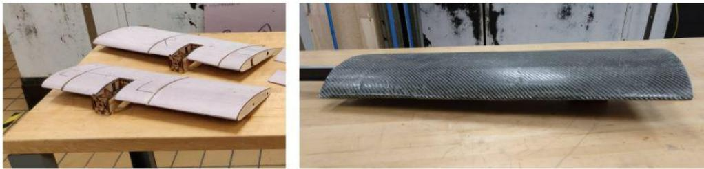
Figure 34: Wings Before and After Composite Layup
