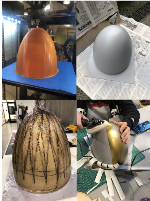
Figure 6.1: (Clockwise from top left): 1. Mold being 3D-Printed, 2. Primed and sanded, 3. Release film applied, 4. Fiberglass layup
