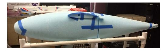
Figure 6.3: CNC-milled fuselage
