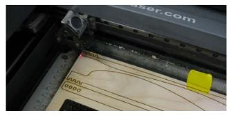
Figure 6.5: Laser cutting of the dropping mechanism
