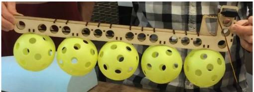
Figure 6.6: Dropping mechanism loaded with plastic balls
