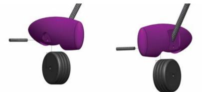
Figure 5.3: Landing gear installation
