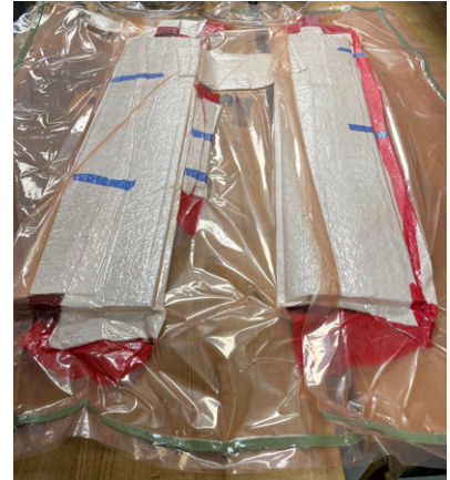
Figure 38: Wings Curing in the Vacuum Bag
